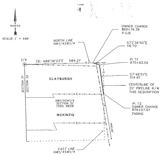
BASIS OF BEARING IS WYOMING STATE PLANE (EAST CENTRAL ZONE) © = FOUND SET STONE
