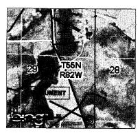
An easement 30 Feet in width, being 15 Feet on each side of the following described line. Commencing at the Southeast Corner of Section 29, T55N, R82W, thence N20°26'20.308"W a distance of 1950 Feet, more or less, to the POINT OF BEGINNING; thence S65°2'36.675"E a distance of 531 Feet, more or less, thus to the ending point.
