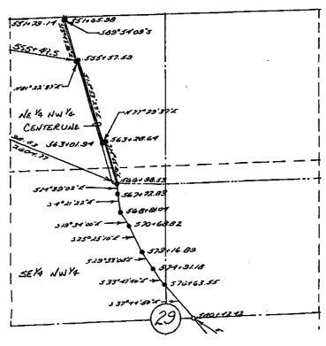
TIE: FROM STA. 566+98.53 N.57°10'01"W 2604.77" TO NW SEC. COR. SEC. 29, T. 54N., R. 83W.
