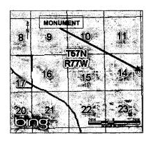
An easement 30 Feet in width, being 15 Feet on each side when measured at right angles to the following described line. Commencing at the East Quarter Corner of Section 14, T57N, R77W located at 44°55'9.043"N, 106°5'43.230"W, thence N89°47'18"W a distance of 18341 Feet, more or less, to the Point of Beginning; thence S51°25'7"W a distance of 356 Feet, more or less, thus to the ending point.
