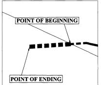
An easement 20 feet in width, being 10 feet on each side when measured at right angles to the following described line. Commencing at the Northwest Corner of Section 27, T57N, R83W, thence S16°23'32"E for a distance of 3414 feet, more or less; to the POINT OF BEGINNING; thence S86°19'34"W for a distance of 205 feet, more or less; thus to the ending point.
