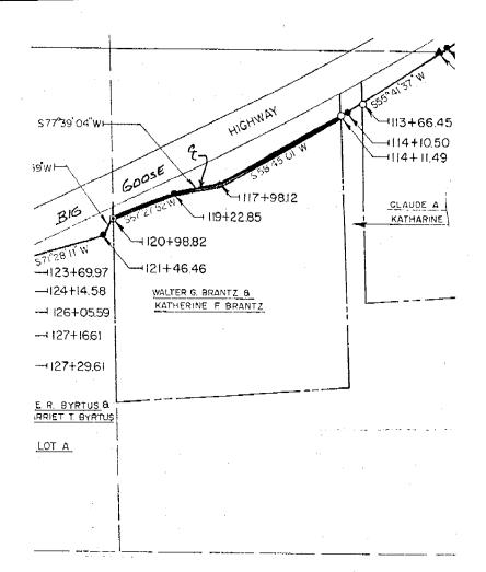
TIES FROM A BRASS CAP AT THE NW COR, OF SECTION 32
