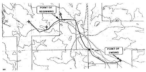
The above description is for a three-phase 24.9/14.4kV single circuit overhead power line "Right-of-Way", 30' in width, being 15' on either side of the described centerline. Right of Way is also provided as required for guys and anchors.
