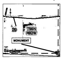
An easement 30 Feet in width, being 15 Feet on each side when measured at right angles to the following described line. Commencing at the South Quarter Corner of Section 29, T55N, R82W located at 44°42'17.254"N, 106°45'34.593"W, thence N54°21'54"W a distance of 2338 Feet, more or less, to the Point of Beginning; thence N11°6'34"E a distance of 263 Feet, more or less, thus to the ending point.
