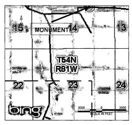
An easement 30 Feet in width, being 15 Feet on each side of the following described line. Commencing at the Center East Sixteenth Corner of Section 14, T54N, R81W, thence S23°6'8.174"W a distance of 7402 Feet, more or less, to the POINT OF BEGINNING; thence S69°42'51.335"E a distance of 411 Feet, more or less, thus to the ending point.
