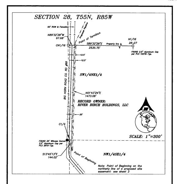
BEARINGS ARE BASED ON THE WYOMING COORDINATE SYSTEM, NAD 1983, EAST CENTRAL ZONE. DISTANCES ARE MULTIPLIED TO SURFACE BY THE ADJUSTMENT FACTOR OF 1.00025.
