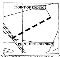
An easement 30 feet in width, being 15 feet on each side when measured at right angles to the following described power line. Commencing at the North West Corner of Section 2, T55N, R83W, thence S52°50'02"E for a distance of 6212 feet, more or less; to the POINT OF BEGINNING; thence N60°56'36"E for a distance of 1195 feet, more or less; thus to the ending point.
