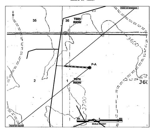
Point P-A is set at the center of a circular tract of land with a radius of 40 feet.
