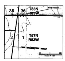
An easement 30 Feet in width, being 15 Feet on each side of the following described line. Commencing at the Northwest corner of Section 1, T57N, R83W, thence S1°28'50"W a distance of 935 Feet, more or less, to the POINT OF BEGINNING; thence S86°23'53"E a distance of 719 Feet, more or less, thus to the ending point.
