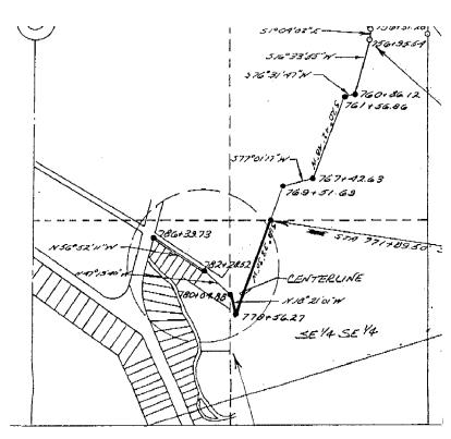
TIE: FROM STA. 771+89.5 N 38° 42'02"E 1681-85' TO E 14 COR. OF SEC. 8 T534R83W
