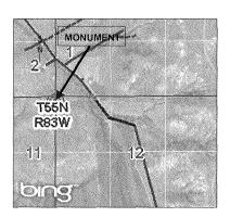
An easement 30 Feet in width, being 15 Feet on each side of the following described line. Commencing at the Northwest corner of Section 12, T55N, R83W, thence S89°40'52.241"E a distance of 974 Feet, more or less, to the POINT OF BEGINNING; thence S35°52'59.676"E a distance of 496 Feet, more or less, thence S75°13'2.677"E a distance of 643 Feet, more or less, thus to the ending point.
