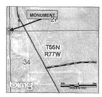
An easement 30 Feet in width, being 15 Feet on each side of the following described line. Commencing at the Northwest Corner of Section 34, T55N, R77W, thence S45°20'24.973"E a distance of 1292 Feet, more or less, to the POINT OF BEGINNING; thence N80°43'55.663"E a distance of 883 Feet, more or less, thence N89°8'26.489"E a distance of 394 Feet, more or less, thus to the ending point.
