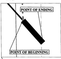
An easement 30 feet in width, being 15 feet on each side when measured at right angles to the following described power line. Commencing at the North East Corner of Section 16, T55N, R78W, thence S01°34'54"E for a distance of 4946 feet, more or less; to the POINT OF BEGINNING; thence S41°10'54"E for a distance of 225 feet, more or less; thus to the ending point.
