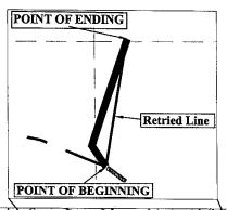
An easement 30 feet in width, being 15 feet on each side when measured at right angles to the following described line. Commencing at the South East Corner of Section 20, T56N, R83W, thence N52°43'59"W for a distance of 10140 feet, more or less; to the POINT OF BEGINNING; thence N33°43'18"W for a distance of 105 feet, more or less, thence N18°17'31"E for a distance of 476 feet, more or less; thus to the ending point.
